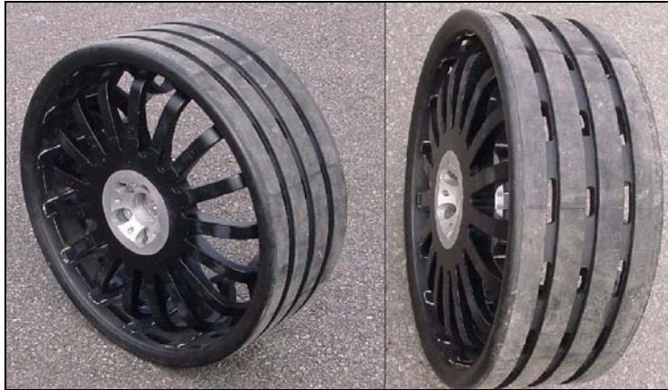
Fig. 53. (above) Early version of a composite wheel (not a good design re. noise). Note the ventilation holes in the tread. New version is underway in which the spokes are better designed to reduce stiffness variations around the circumference and with better distributed ventilation holes.
