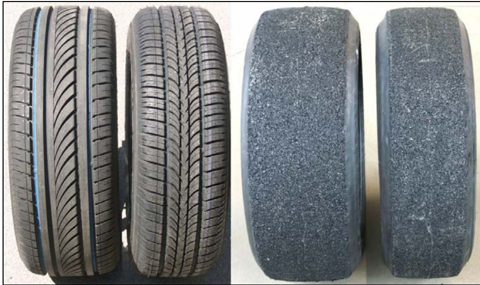
Fig. 56. Two porous tread tyre prototypes together with the regular tyres used as carcasses for the porous tread (after buffing-off the existing tread).
