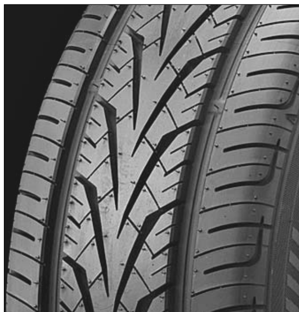
Fig. 47 (left). The Yokohama AVS dB S2 tyre; one of the quietest tyres on the market, which seems to combine the principles outlined in Fig. 46 and Fig. 48.
