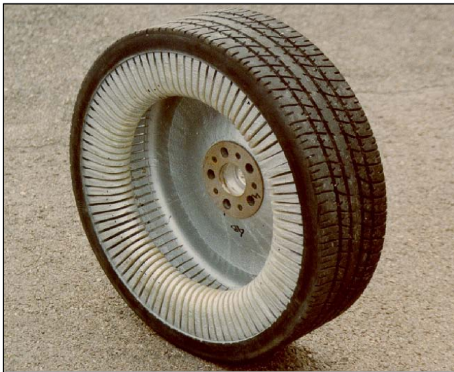
Fig. 55. Composite wheel, invented by H E Hansson, tested by VTI in 1991, see Table 25.1 in [Sandberg & Ejsmont, 2002]. The Michelin Airless tyre somewhat resembles this design.
