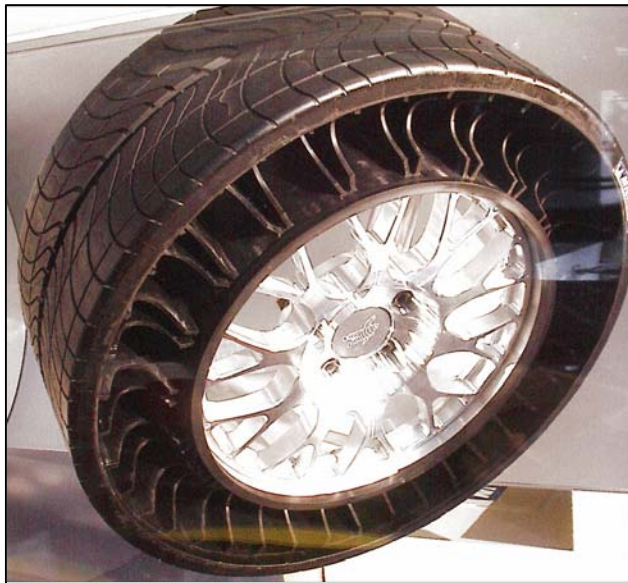
Fig. 53. (above) Early version of a composite wheel (not a good design re. noise). Note the ventilation holes in the tread. New version is underway in which the spokes are better designed to reduce stiffness variations around the circumference and with better distributed ventilation holes.
