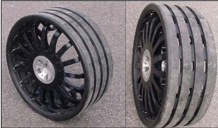
Figure 4.15: Early version of a composite wheel. Note the ventilation holes in the tread. New version is underway in which the spokes are better designed to reduce stiffness variations around the circumference and with better distributed ventilation holes
