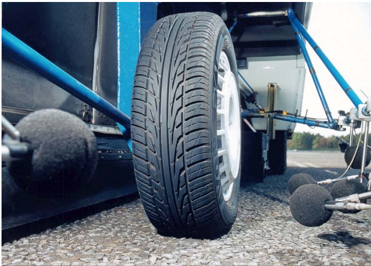
Figure 6.8: Test tyre and microphone set-up in TRITON's enclosure
