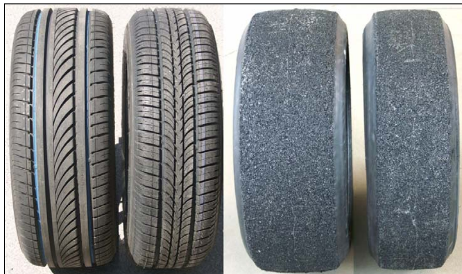
Figure 4.17: Two porous tread tyre prototypes together with the regular tyres used as carcasses for the porous tread (after buffing-off the existing tread)
